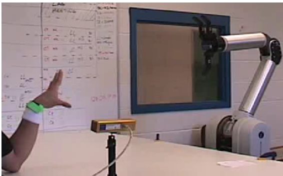
Fig. 4. Embodied interaction study: Subjects play the shadow puppet game with our 4 DOF Whole Arm Manipulator (WAM). A stereo camera is used to code the gestural language tokens of the human in real-time.
